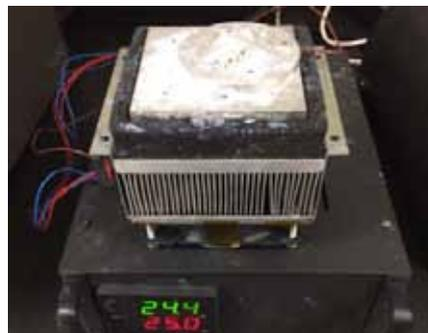
Figure 1: Peltier-based thermal performance analyser
