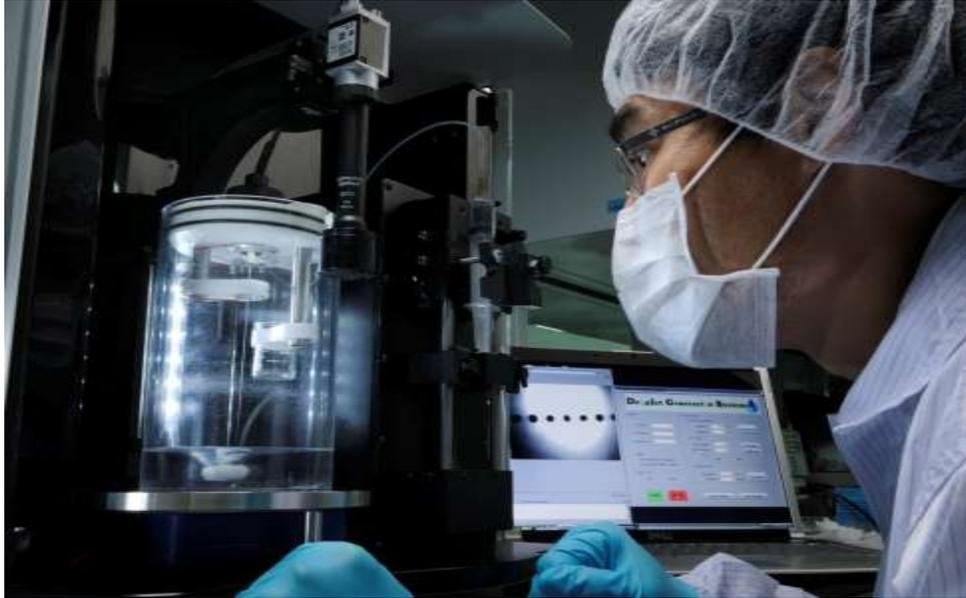
*Picture 2: The SIMTech microfluidic-based droplet generation technology allows high throughput and contamination-free microencapsule formation of cells, enzymes or drug.*
